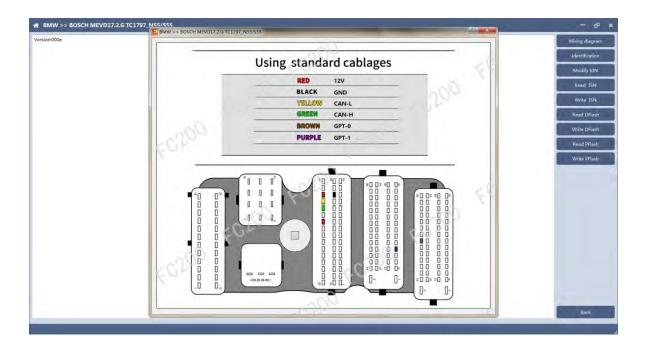
Click the "Wiring Diagram" button to view the ECU wiring diagram, connect the wiring harness correctly according to the wiring diagram, and connect with FC200, plug in DC12V interface of FC200 with 12V power supply.
