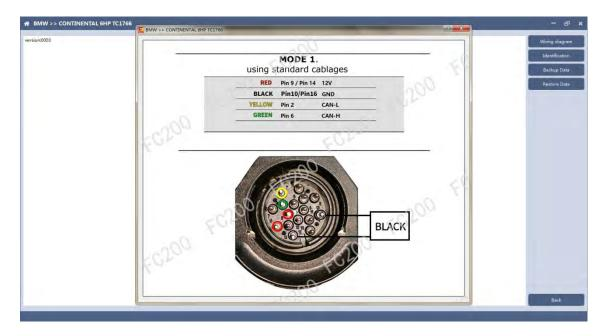
Click the "Wiring Diagram" button to view the ECU wiring diagram, connect the wiring harness correctly according to the wiring diagram, and connect with the device, plug in the device DC12V interface with 12V power supply.
